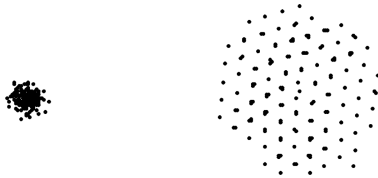
Fig. 4: Initially, the particles are assumed to be in a tight cluster t = 0 (left). Then particles repel, and after 1,000 time steps form a good hexagonal lattice (right).
